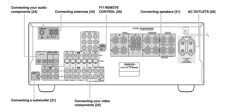
Here is an explanation of typical ways to connect various components to the TX-SR700/700E. There are many ways that any one component can be connected, and it is up to you to decide which method best fits your situation. The directions given here are only one option and should only be thought of as such. It is best to fully understand the nature of each connector and terminal as well as those of your components and their features to ascertain which method of connection is best.
